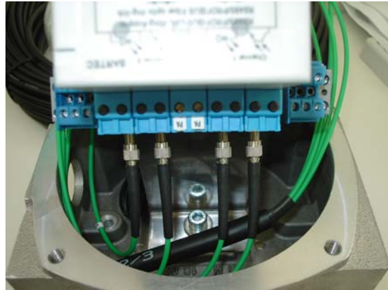
- Connection with fibre optic interface – terminals - Connection with fibre optic interface – fibre optic cable
