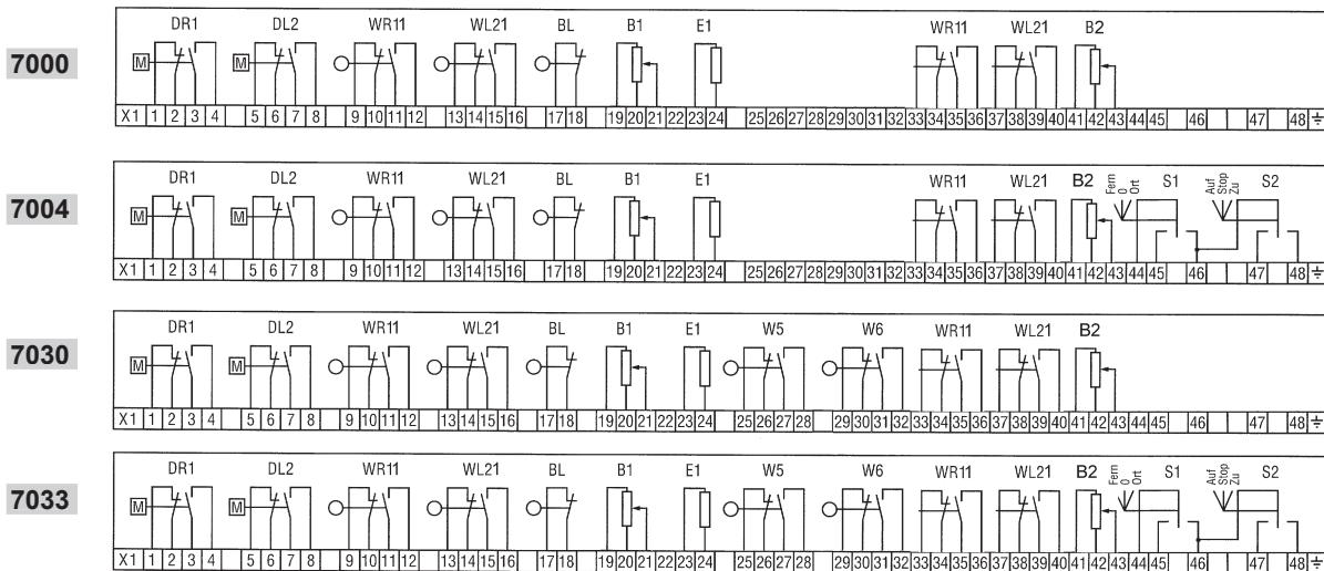
Basic equipment with electronic position transducer B 3, heater E 1 and variants
