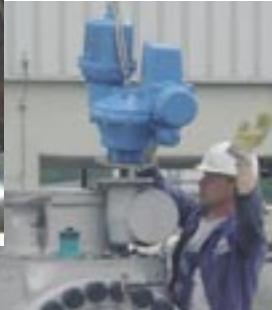
We offer the service of valve measuring, actuator sizing and mounting actuators by means of special adaptors to the existing valve interface. This kind of service has even to be considered strongly on automation and rehabilitation projects if for example the valve cannot be replaced from the pipe, long delivery times delay the project, or costs for a new valve plus actuator exceed the effect saved by the automation.
